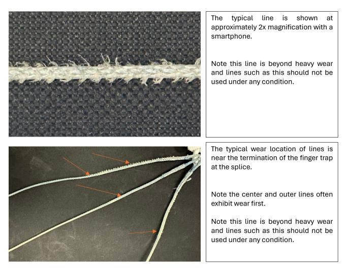
A line plan should be obtained from the manufacturer for this inspection. The lines/items listed in **bold** are critical and should NEVER be jumped with wear at heavy condition. We suggest that critical lines be replaced when wear is at/or beyond medium.
