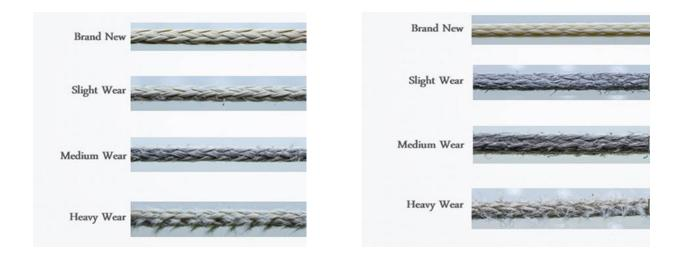
Lines should be evaluated for *slight/medium/heavy* wear conditions. Lines identified as critical should be replaced prior to the heavy wear condition.
