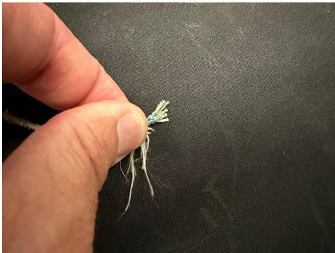
Photograph 7: View of angled cut at failed line.
