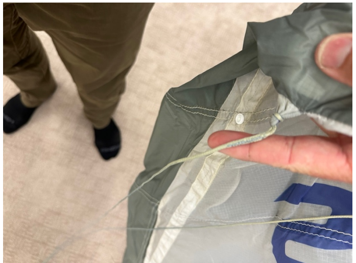
Photograph 8: View of wear at upper portion of lines.
