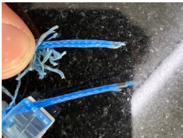
Photograph 16: View of line cut at angle on interior of splice.
